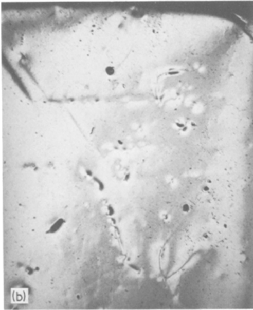
Figure 3 Optical micrographs imaged using Nomarski interference contrast at \times 60 for a \langle 001 \rangle axis specimen deformed at 0.56T_m at 10^{-5} \text{ sec}^{-1} , (a) as-deformed, (b) above area chemically polished in a bromine-methanol solution, (c) above area etched in boiling 6:6:1 ( \text{HNO}_3 : \text{H}_2\text{O} : \text{HCl} ).
