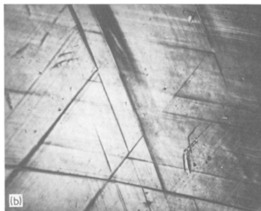
Figure 2 Optical micrographs imaged using Nomarski interference contrast at \times 150 showing (a) fine slip on the \{1\ 4\ 5\} face of a \langle 1\ 2\ 3 \rangle axis specimen deformed at 0.67T_m at 10^{-4} \text{ sec}^{-1} ; (b) Deformation twins on the \{1\ 1\ 0\} face of a \langle 0\ 0\ 1 \rangle axis specimen deformed at 0.61T_m at 10^{-5} \text{ sec}^{-1} .
